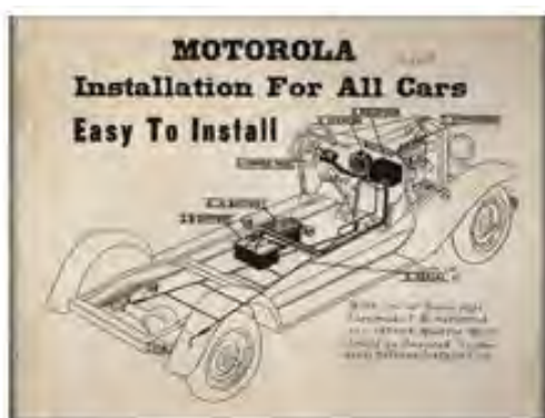
A Motorola car radio installation diagram (circa 1930) showed batteries, spark plug suppressors and the antenna, in addition to the radio components.
